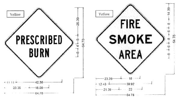
Temporary Traffic Control Warning signs to be used when roadway visibility has been restricted by smoke. A roll up REDUCE SPEED sign made of retroreflective incident management pink roll up vinyl may be used now, as it will eventually replace the REDUCE SMOKE SPEED orange mesh sign. No new mesh signs are to be manufactured.
