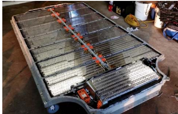
Tesla battery platform
